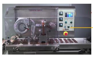
New control of the heating zones, for more precision Touch screen with:
